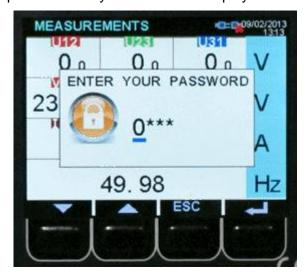
A 4 digit password must be entered using and buttons. The factory default password is "9876". The buttons modify the value of the current digit. The button steps to the next digit.
