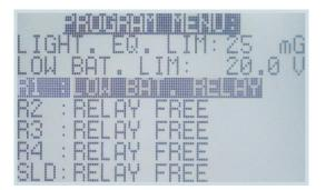
Modified parameters are saved to a non-volatile memory and are not affected by energy failures.
