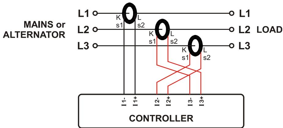
The utility mains is still loaded with 100 kW on each phase. PF in phases L2 and L3 will show -0.50 due to phase shift between voltages and currents which is caused by CT swapping. As a result, the total power displayed will be 0 kW.
