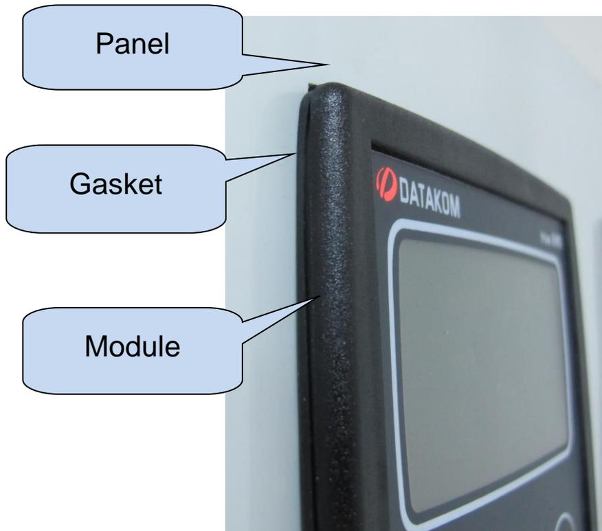
The rubber gasket (sold separately) provides a watertight means of mounting the module to the panel. With the gasket, IEC 60529-IP65 protection is provided. A short definition of IP protection levels is given below:
