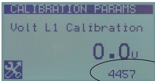
right of the screen, and press
