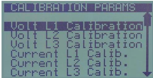
The unit is calibrated before it leaves the factory, but it is possible to recalibrate.
