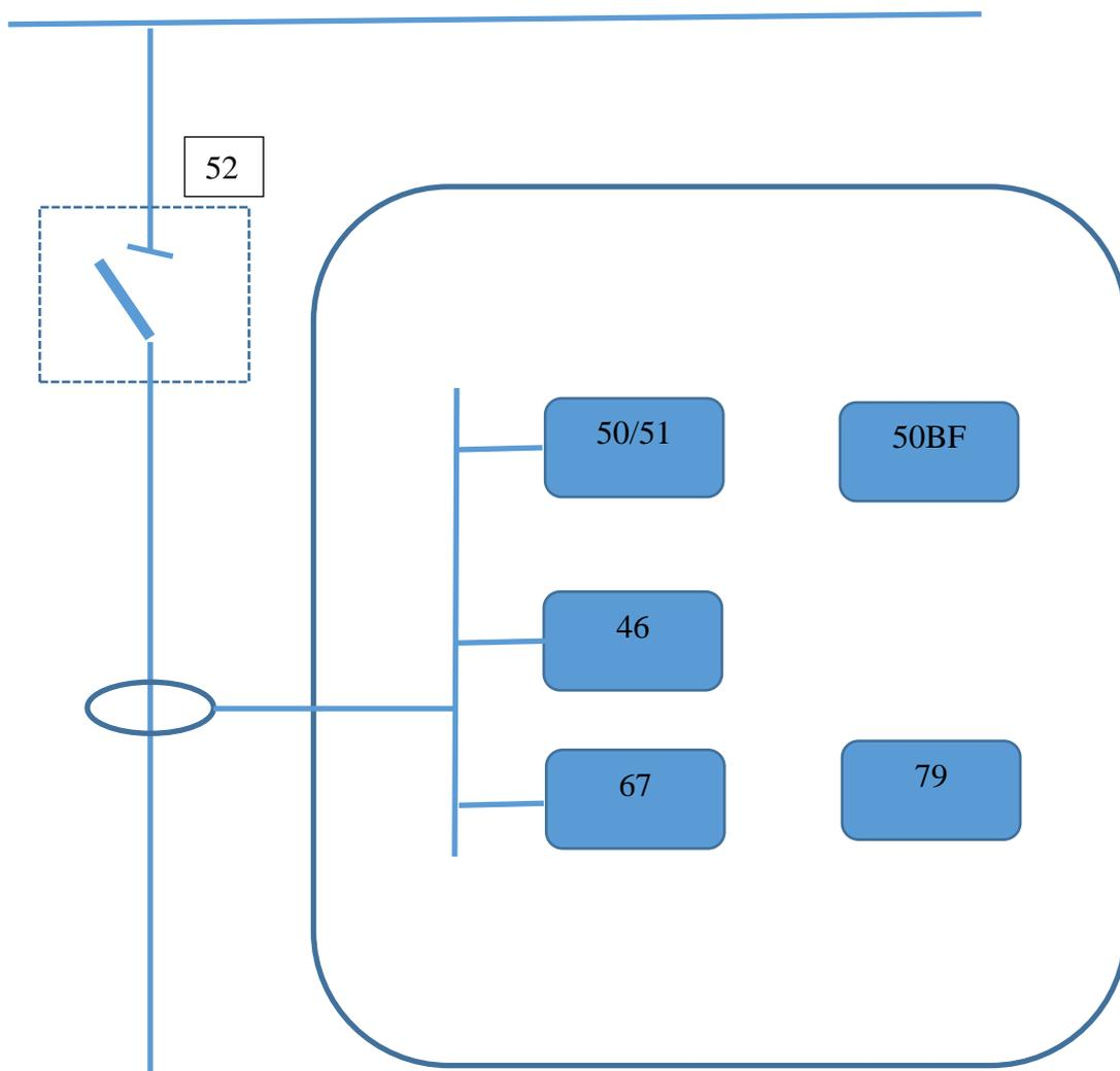
DPR350 allows for two levels of “Overcurrent Protection” and “Negative Sequence Overcurrent Protection” functions.
