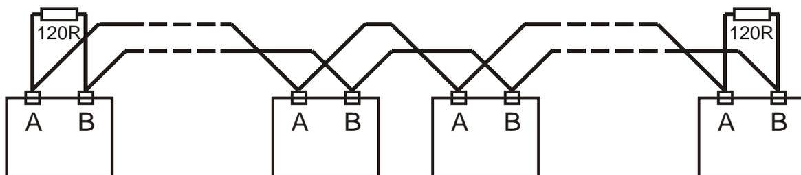
The line must be terminated by 120 ohms on each end.
