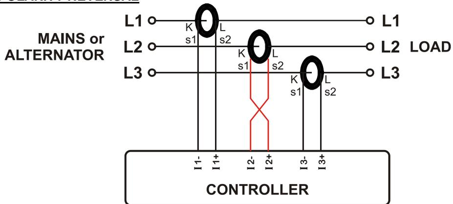
The utility mains is still loaded with 100 kW on each phase. The load power factor (PF) on Phase L2 will show -1.00 due to reverse CT polarity. As a result, total load power displayed will be 100 kW.
