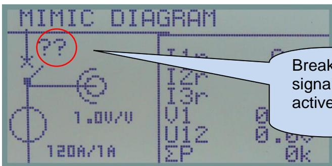
Breaker open with correct open input signal, but breaker open input signal also active.
