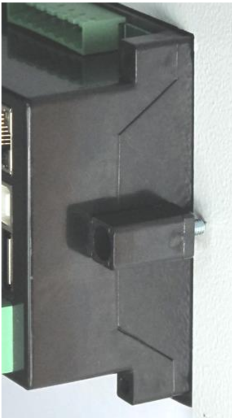
Installation of screw type bracket
