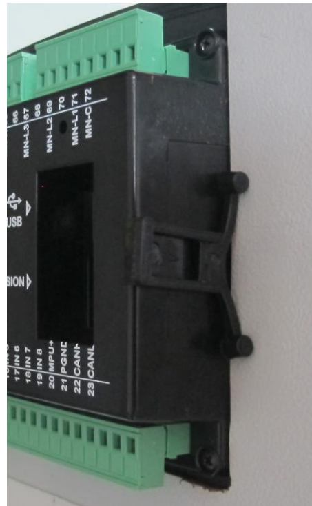
Installation of self retaining type bracket
