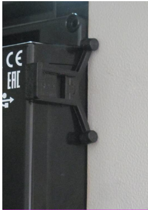
Installation of self-retaining type bracket
