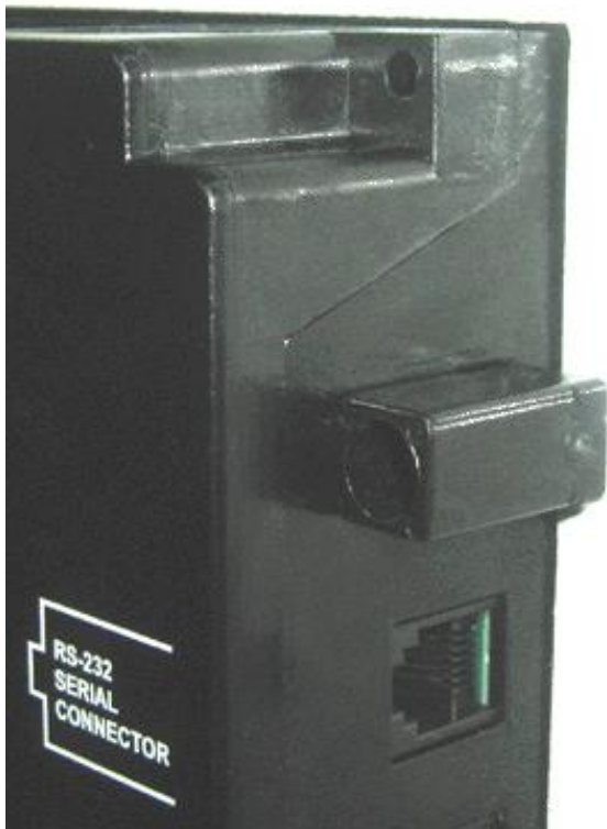
Installation of screw type bracket
