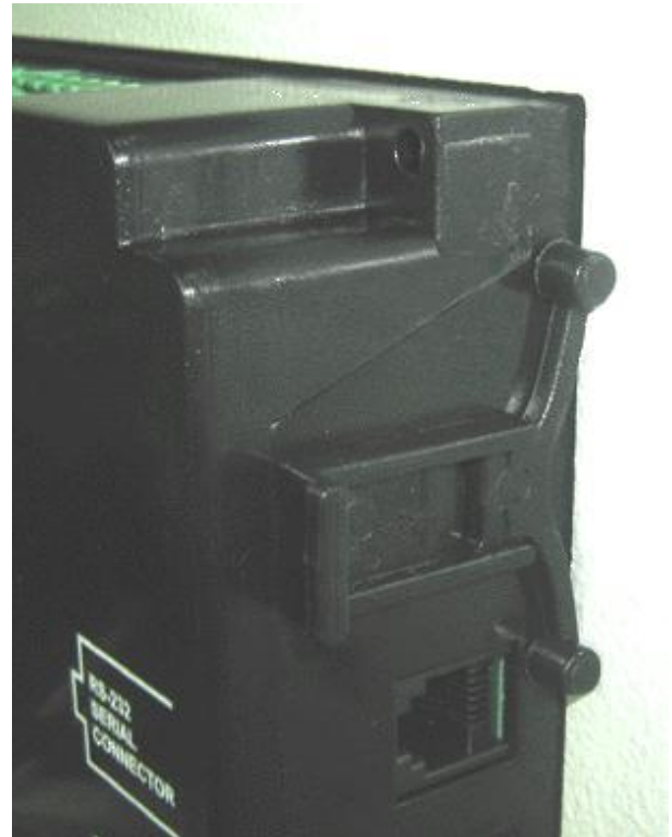
Installation of self retaining type bracket
