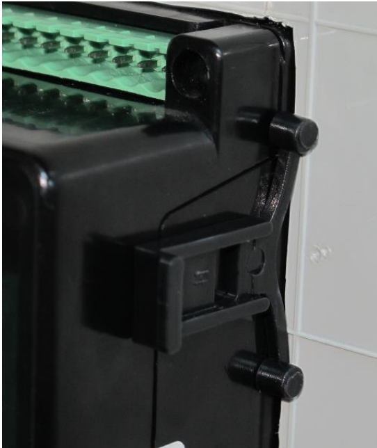
Installation of self-retaining type bracket
