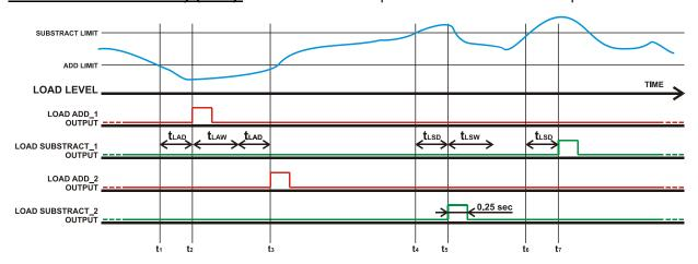
t1: the load goes below the Multi Load Add Power Level.
